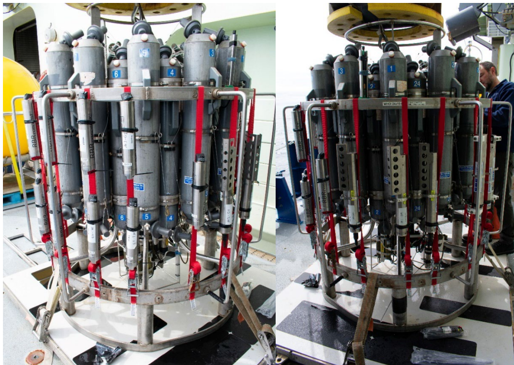
Photos: caldip set up. We felt having optodes ‘upside-down’ would not be an issue during the duration of a cast, and this placement allowed more instruments on the frame and not interacting with ratchet straps.
